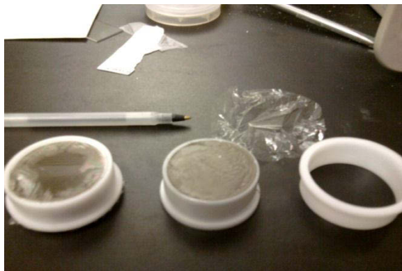
Figure 50: Sample sealing involving pasting a thin film on the surface of the paste
